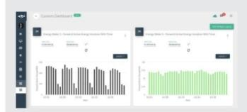
It has feature to show visual alerts in-case a particular value (current, power, power factor) is out of desired ranges. (Pic: Kwh Trend comparison of two energy meters, Realtime tables with visual alerts)
